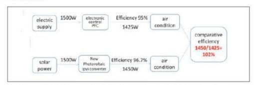
By adopting optimized circuit design and improved software , efficiency of the air-cons improves from 85% to 96.7%!
