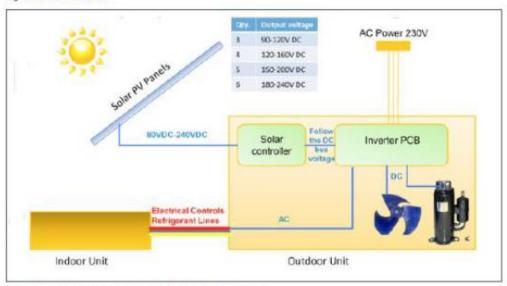
The PCB controller automatically gives priority to solar power!
